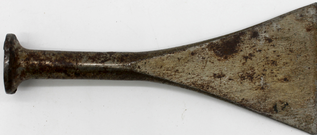
A caulking iron, used by shipwrights to assist with hammering oakum into the seams between planks on ships, 2025.3.1
